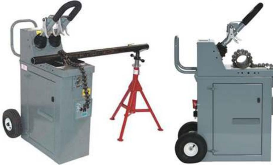
The Kwik-Snap™ 2500 Production Cast Iron Soil Pipe Cutter is a powerful portable high volume soil pipe cutter for cast iron pipe. With its 3.5 second cutting cycle time from the electric hydraulic power, you can cut more pipe faster to get the job done quickly. It has a capacity of 1-1/2" to 6.00" OD pipe and its unique chain design cuts pipe fast, thus eliminating the need to reset for each cut on the same size pipe. It is quiet and reliable and easy to use.
